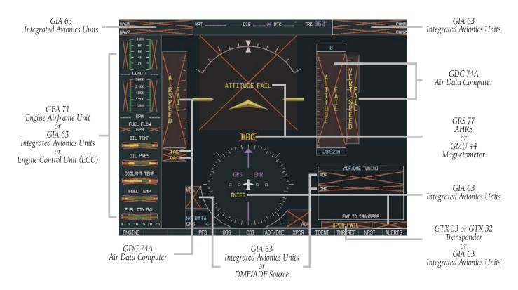
Figure 4 G1000 System Failure Indications
