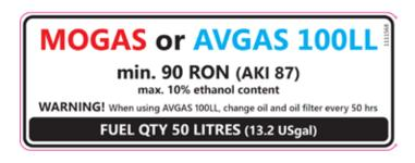
WARNING! When using AVGAS 100 LL, change oil and oil filter every 50 hrs
