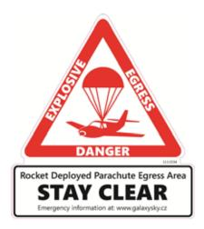
Next to rocket exhaust (bottom of fuselage):
