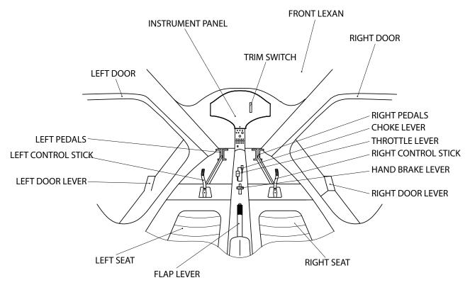
Individual control levers: pilot stick and rudder pedals
